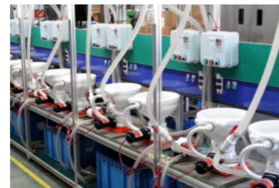
Toilet Lifespan Test Bench
